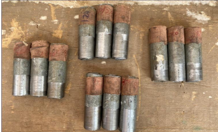
Fig. 5.: All the completed EN19 Steel. workpiece after turning
